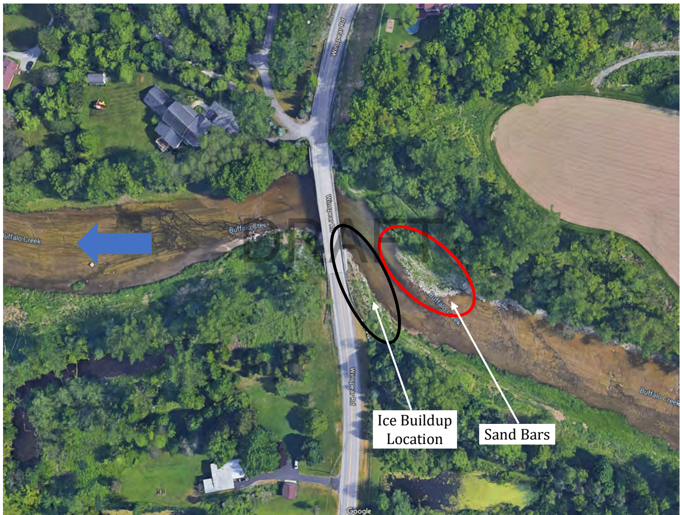
Figure 10. Ice buildup and sand bar locations upstream the Winspear Road bridge in the Town of Elma, NY.
