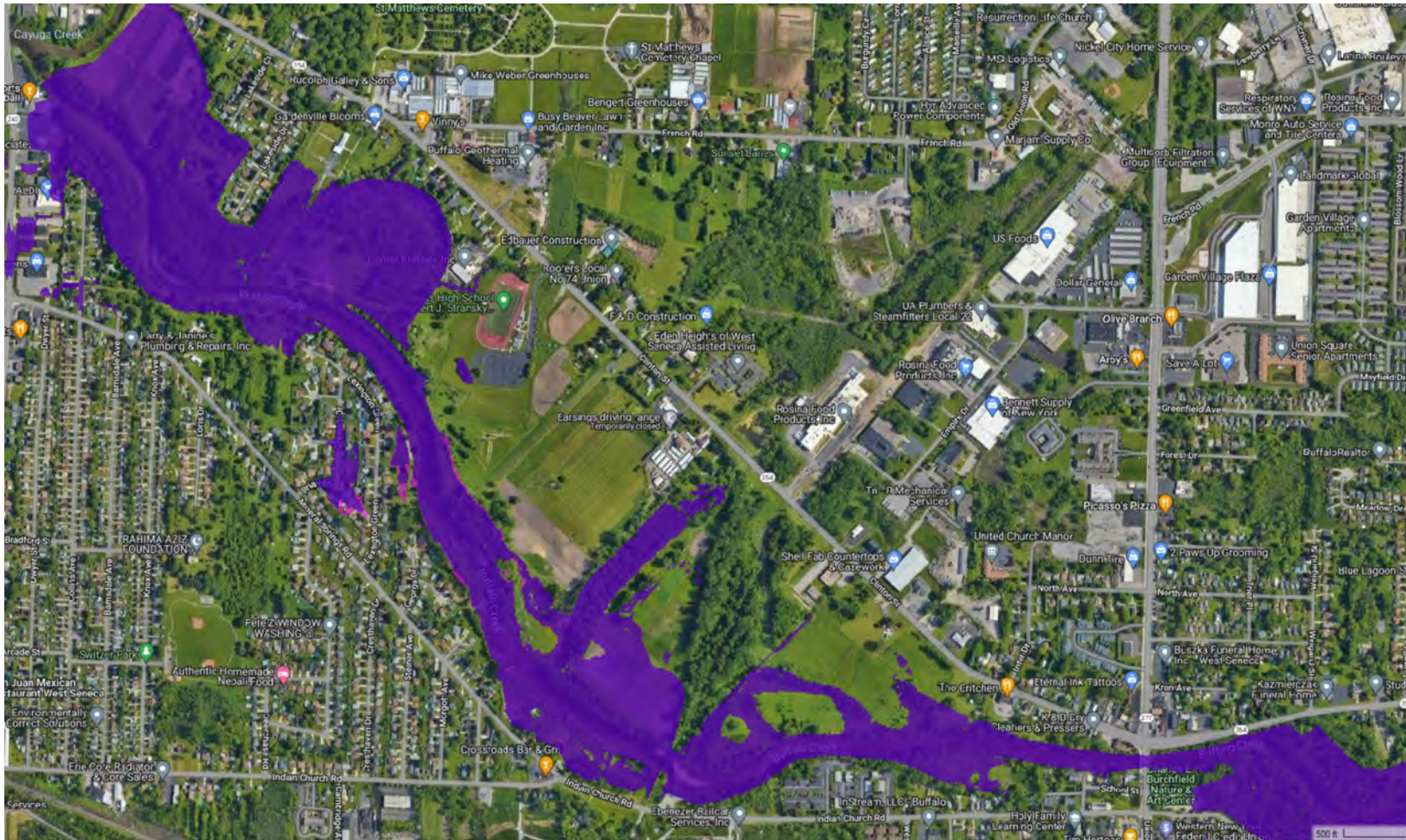
Figure 9. Scenario #1 - Flood extents for proposed conditions (blue) and existing condition (pink) model using the USGS StreamStats 1-percent AEP (100-year recurrence) event peak discharge.
