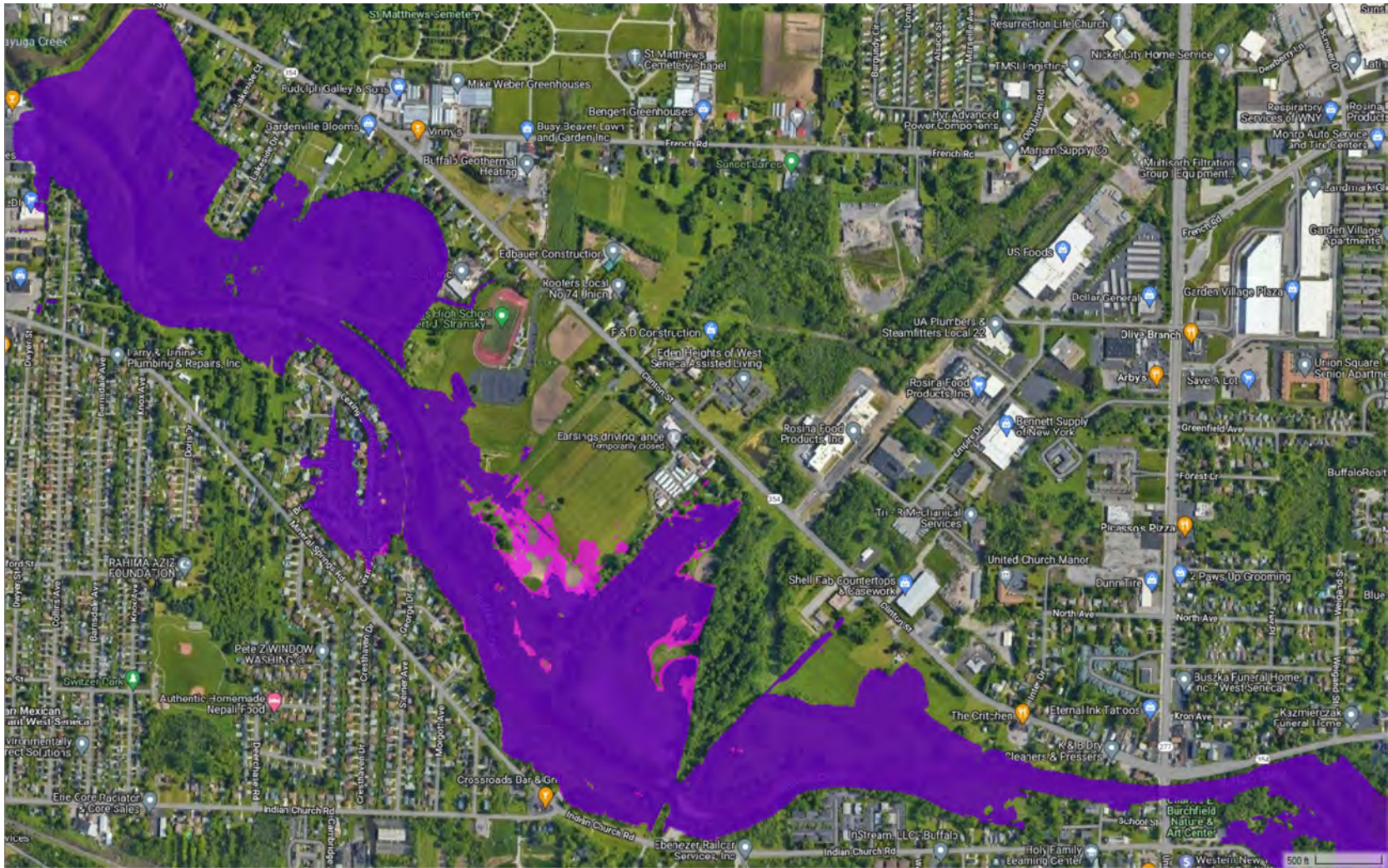
Figure 27. Scenario #8 - Flood extents for proposed (blue) and existing condition (pink) with ice-jam models using the USGS StreamStats 10-percent AEP (10-year recurrence) event peak discharge.
