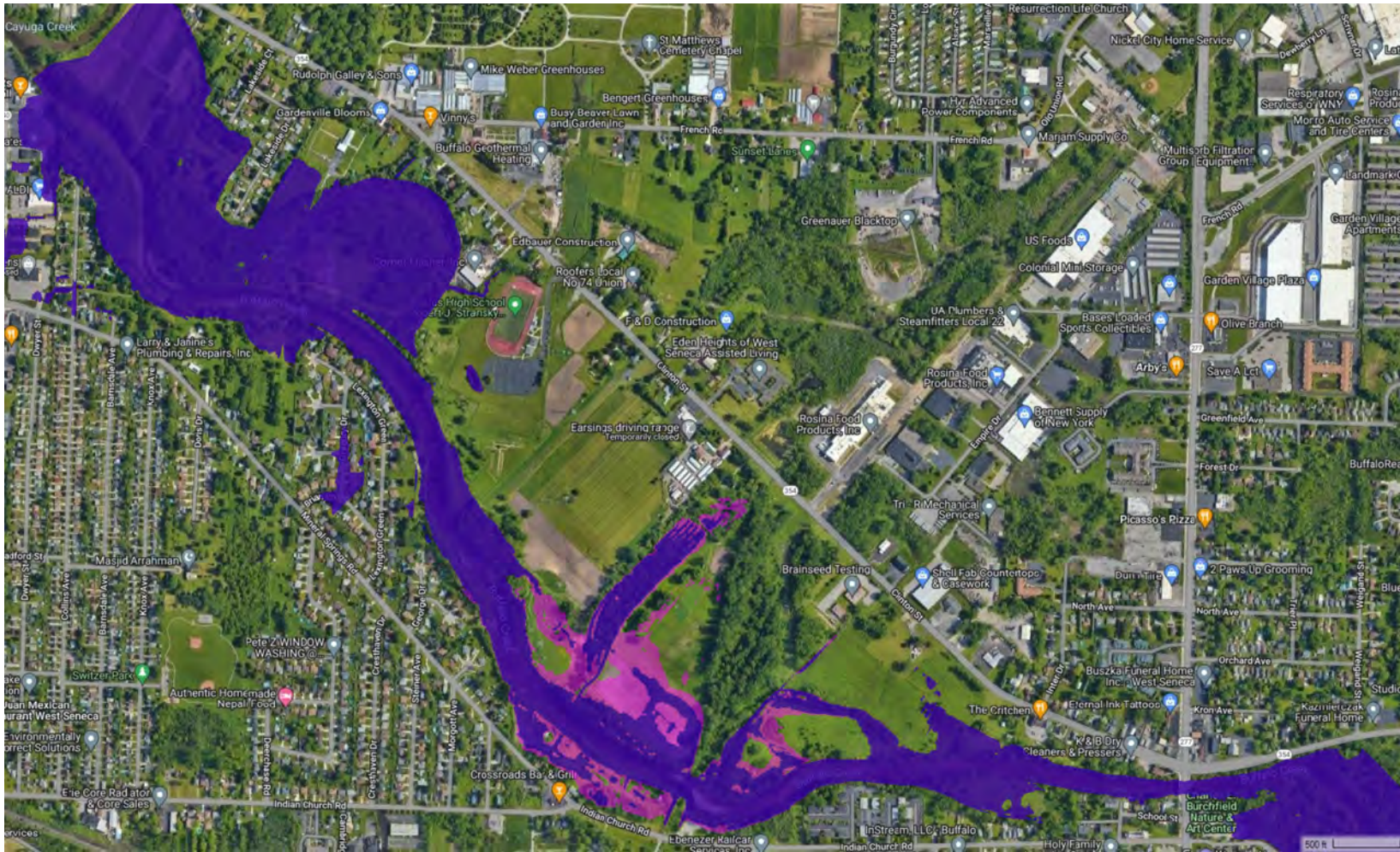
Figure 14. Scenario #6 - Flood extents for proposed (blue) and existing conditions (pink) model using the USGS StreamStats 1-percent AEP (100-year recurrence) event peak discharge.
