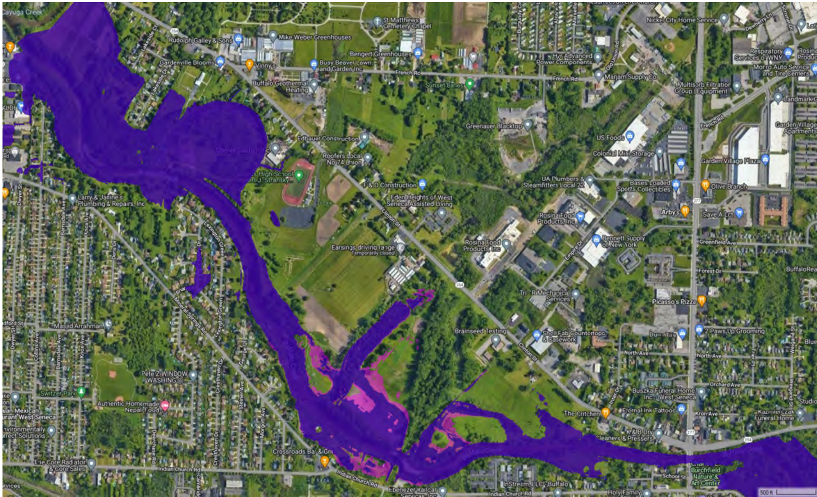
Figure 12. Scenario #4 - Flood extents for proposed (blue) and existing conditions (pink) model using the USGS StreamStats 1-percent AEP (100-year recurrence) event peak discharge.
