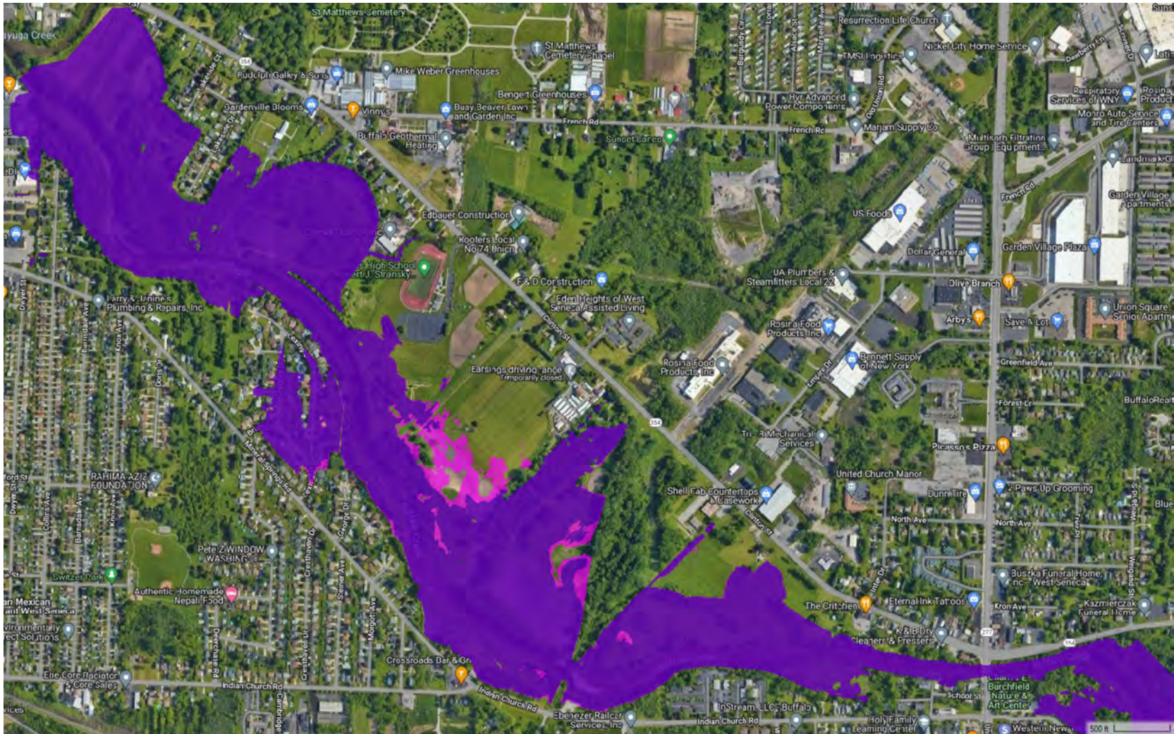
Figure 23. Scenario #4 - Flood extents for proposed (blue) and existing condition (pink) with ice-jam models using the USGS StreamStats 10-percent AEP (10-year recurrence) event peak discharge.
