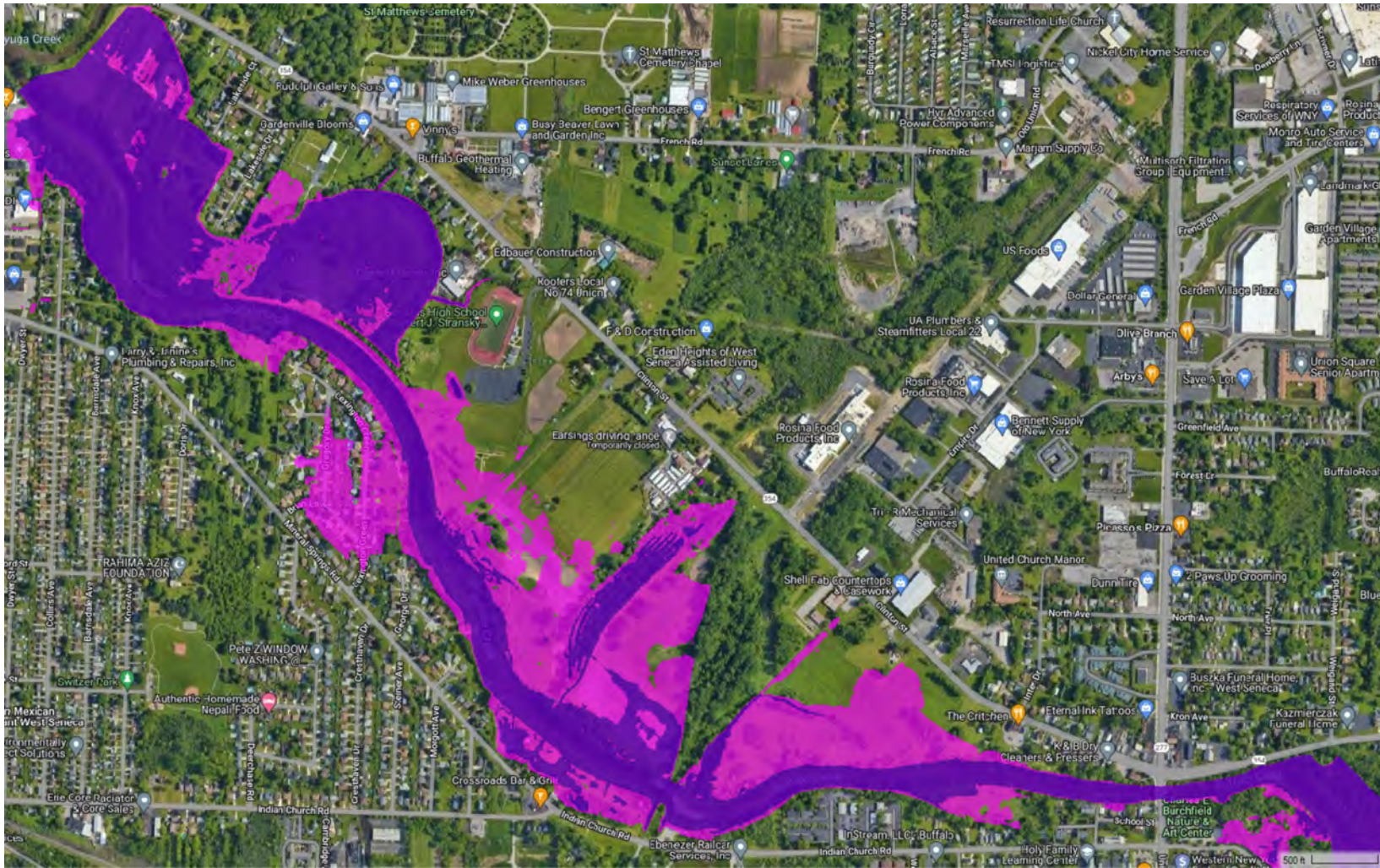
Figure 19. Flood extents for the existing conditions model under open-water (blue) and ice-jam (pink) conditions models using the USGS StreamStats 10-percent AEP (10-year recurrence) event peak discharge.
