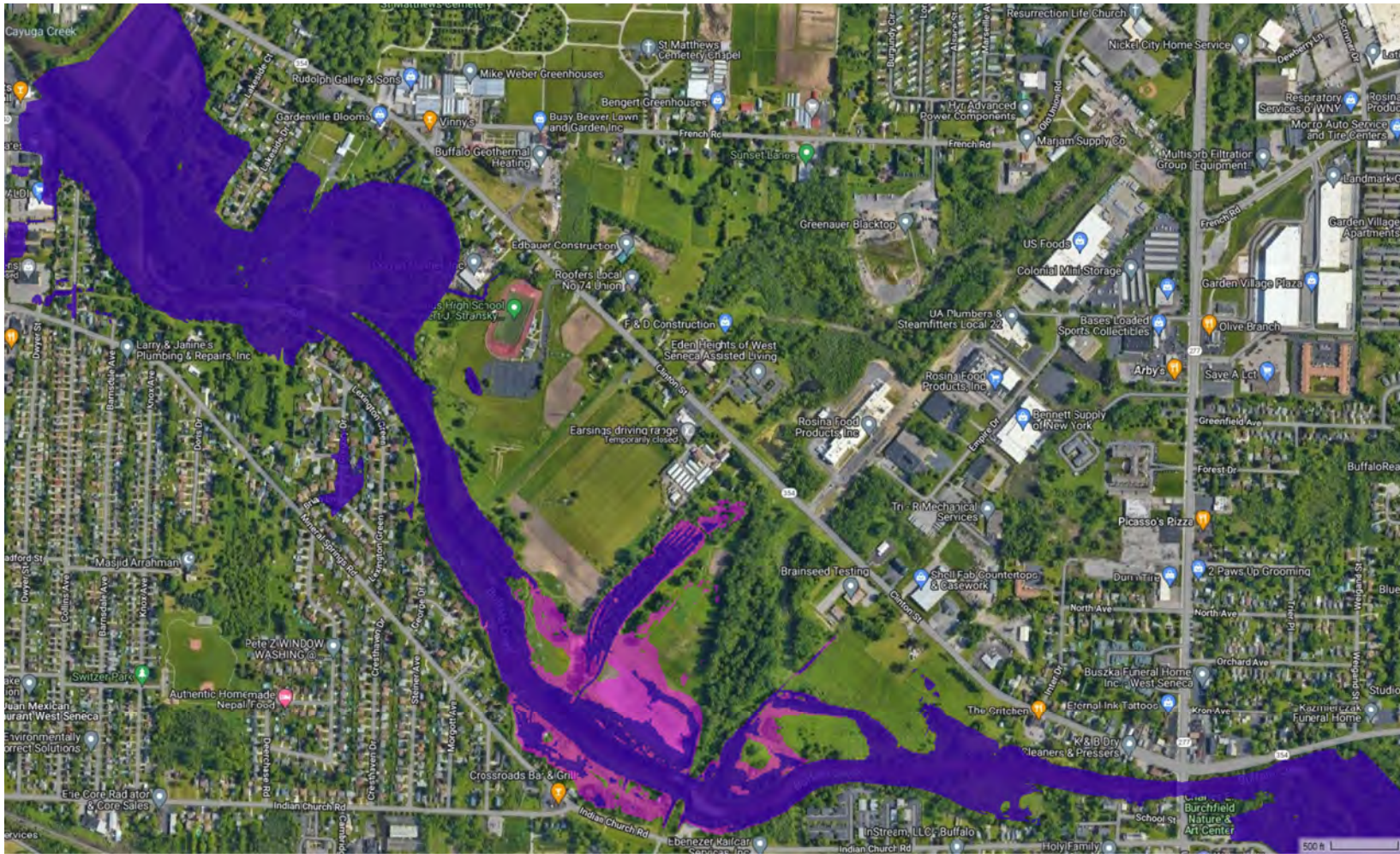
Figure 17. Scenario #9 - Flood extents for proposed (blue) and existing condition (pink) model using the USGS StreamStats 1-percent AEP (100-year recurrence) event peak discharge.
