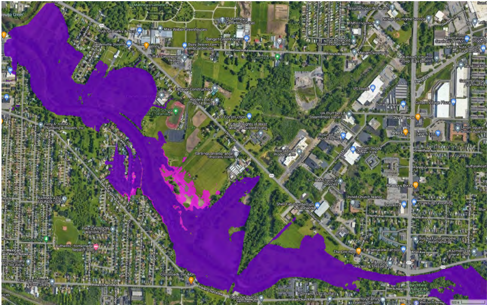
Figure 22. Scenario #3 - Flood extents for proposed (blue) and existing condition (pink) with ice-jam models using the USGS StreamStats 10-percent AEP (10-year recurrence) event peak discharge.
