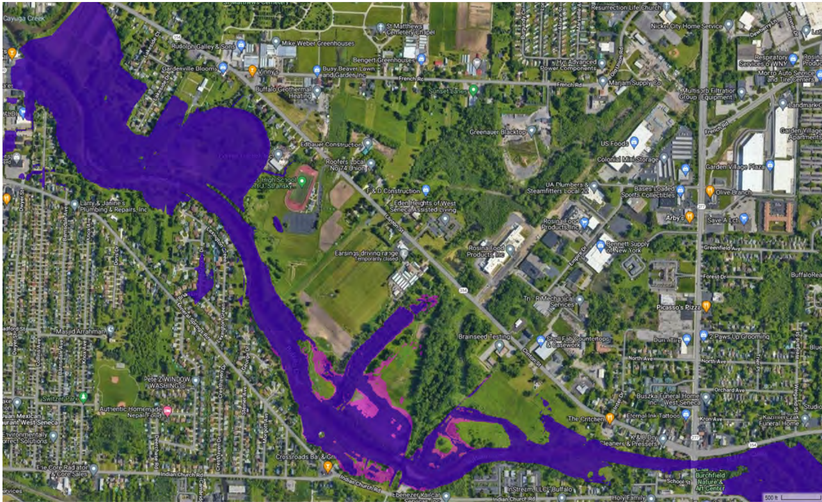
Figure 13. Scenario #5 - Flood extents for proposed (blue) and existing (pink) model using the USGS StreamStats 1-percent AEP (100-year recurrence) event peak discharge.
