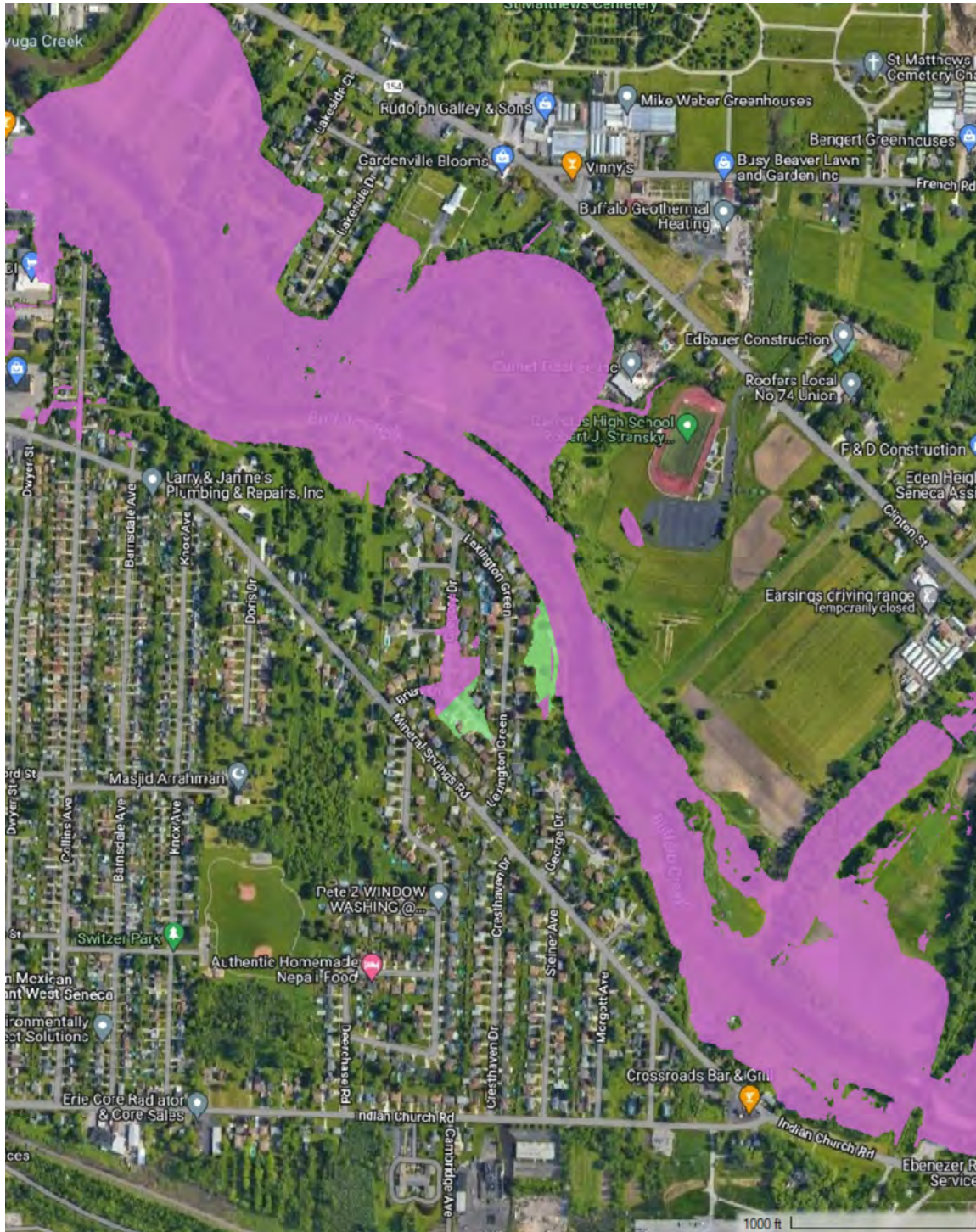
Figure 18. Flood extents for existing with berm (pink) and existing without berm (green) conditions models using the USGS StreamStats 1-percent AEP (100-year recurrence) event peak discharge.
