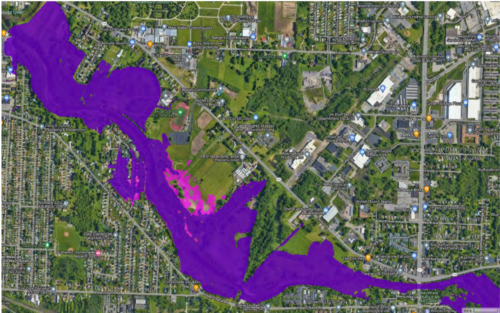
Figure 21. Scenario #2 - Flood extents for proposed (blue) and existing condition (pink) with ice-jam models using the USGS StreamStats 10-percent AEP (10-year recurrence) event peak discharge.
