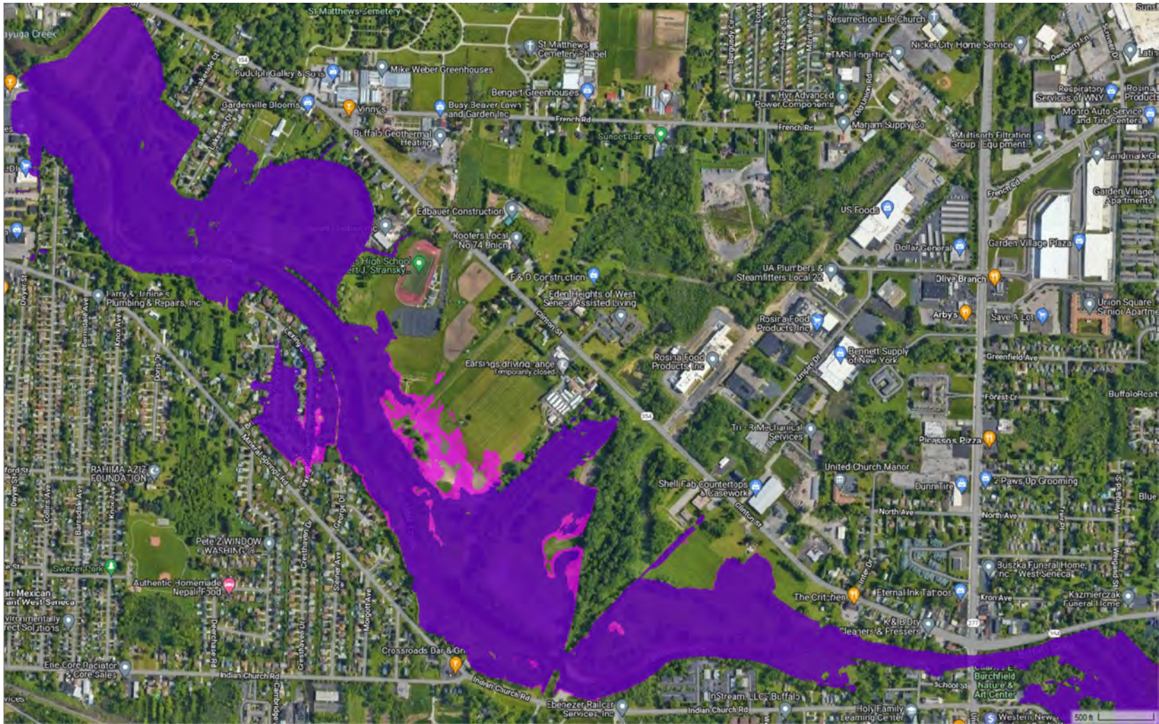
Figure 24. Scenario #5 - Flood extents for proposed (blue) and existing condition (pink) with ice-jam models using the USGS StreamStats 10-percent AEP (10-year recurrence) event peak discharge.
