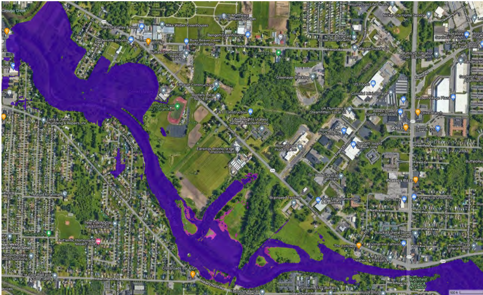
Figure 16. Scenario #8 - Flood extents for proposed (blue) and existing (pink) model using the USGS StreamStats 1-percent AEP (100-year recurrence) event peak discharge.
