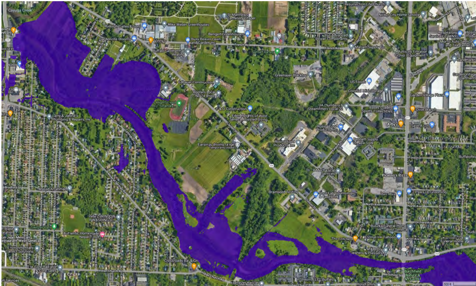
Figure 10. Scenario #2 - Flood extents for proposed (blue) and existing conditions (pink) model using the USGS StreamStats 1-percent AEP (100-year recurrence) event peak discharge.
