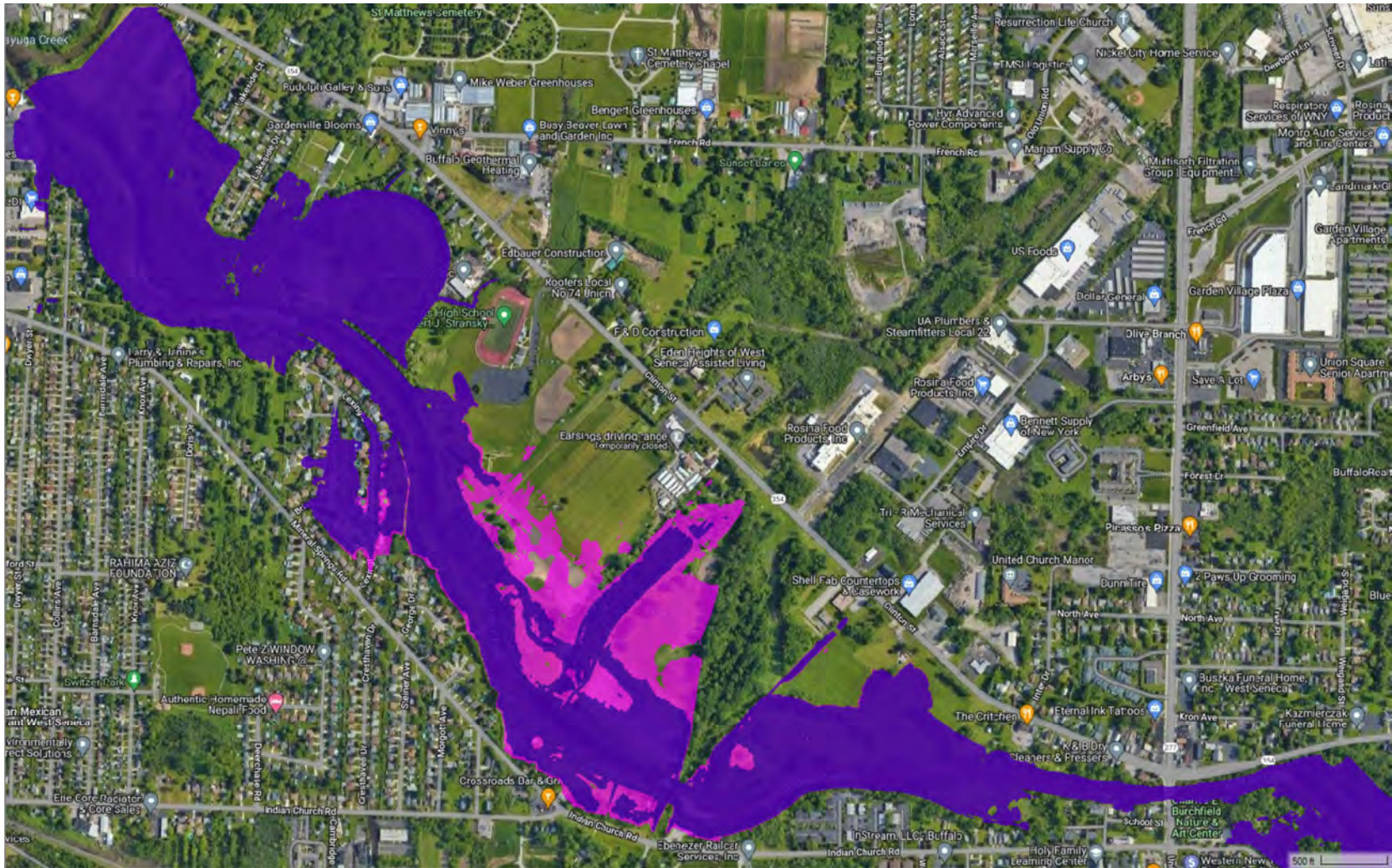
Figure 28. Scenario #9 - Flood extents for proposed (blue) and existing condition (pink) with ice-jam models using the USGS StreamStats 10-percent AEP (10-year recurrence) event peak discharge.
