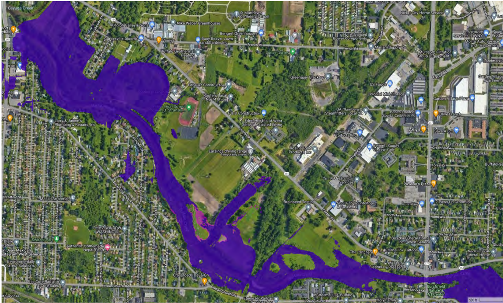
Figure 11. Scenario #3 - Flood extents for proposed (blue) and existing conditions (pink) model using the USGS StreamStats 1-percent AEP (100-year recurrence) event peak discharge.
