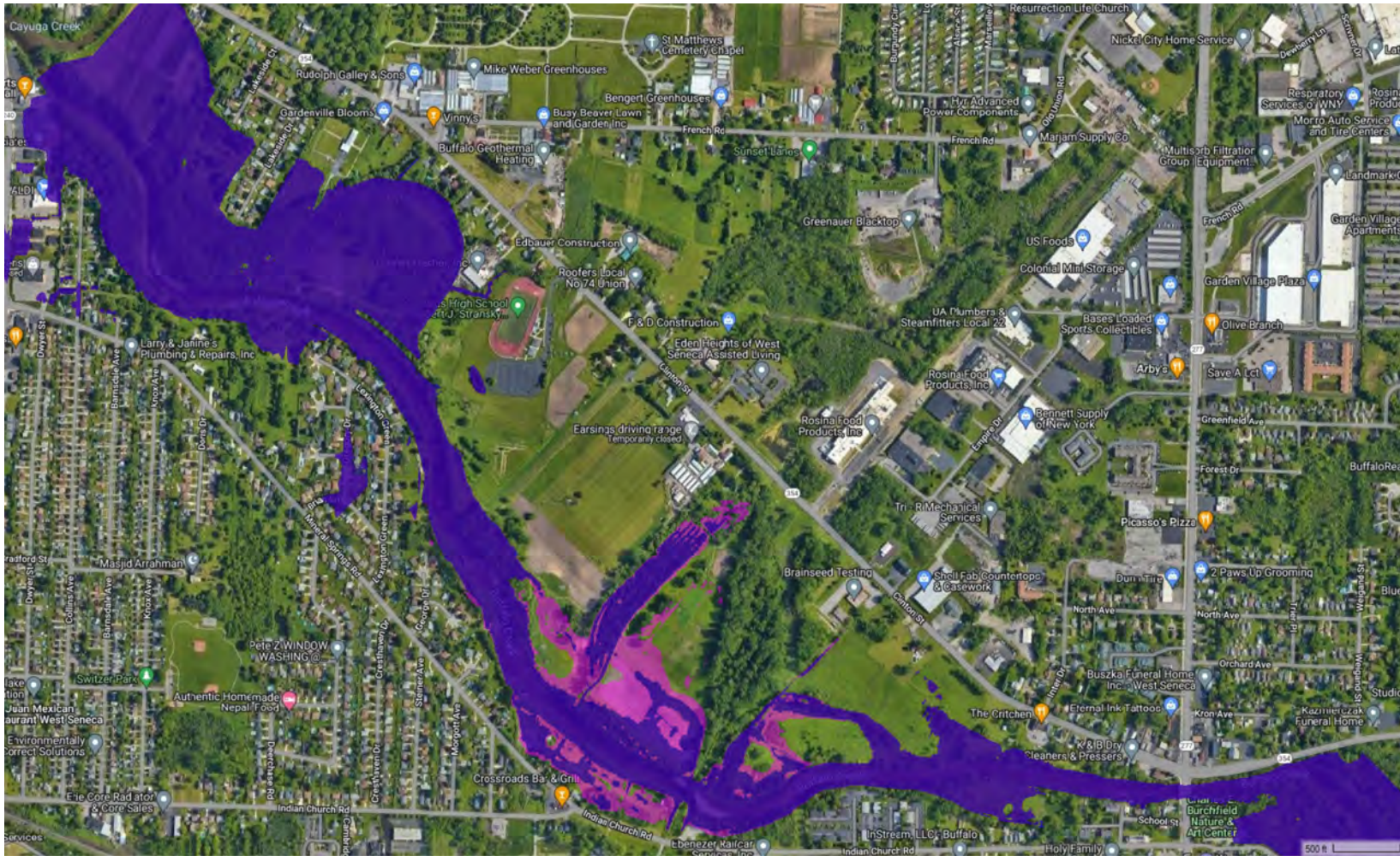
Figure 15. Scenario #7 - Flood extents for proposed (blue) and existing conditions (pink) model using the USGS StreamStats 1-percent AEP (100-year recurrence) event peak discharge.
